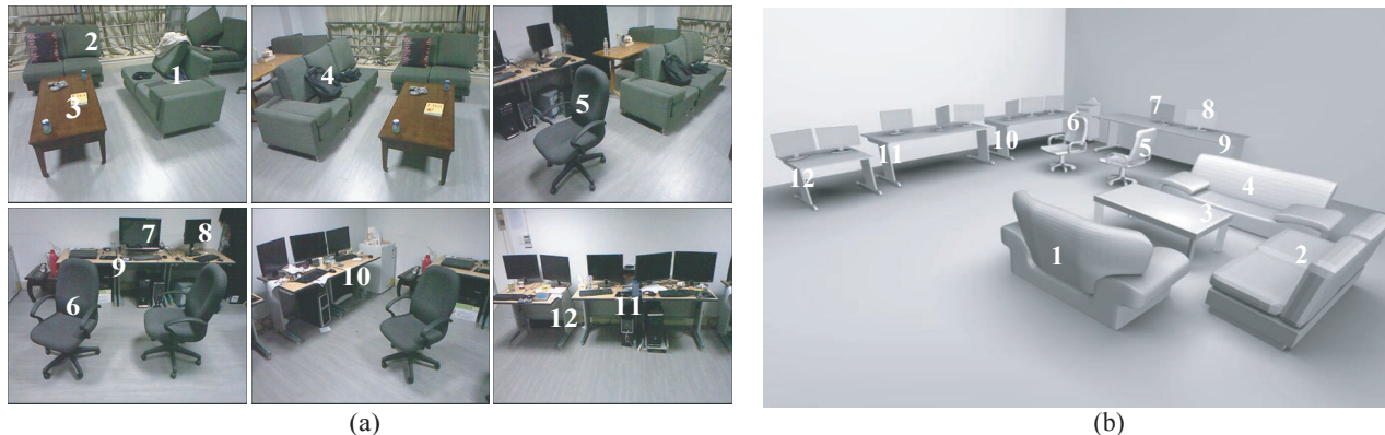
Figure 1: Lab scene. (a) Captured images (Only RGB data are shown). (b) Reconstruction result. Only 6 RGBD images captured by Microsoft Kinect camera are enough for our system to reconstruct its prototype scene with 20 objects of semantic labels (eight monitors are not numbered to avoid possible clutter). The numbers in white indicate the correspondence between objects in the image and their reconstruction results and the overall modeling time of this lab scene is less than 18 minutes.
