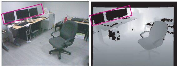
Figure 10: A depth data missing case. Due to the polarization effect in liquid crystal display, it is possible for Microsoft Kinect camera to miss the depth data of the three monitors in the RGBD image.
